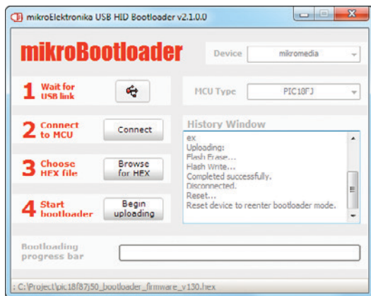
Figure 3-8: mikroBootloader ready for next job
