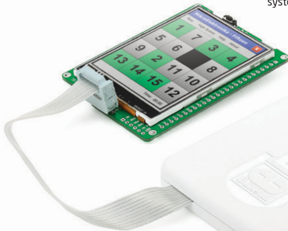
Figure 3-9: Connecting mikroProg™ to mikromedia™
