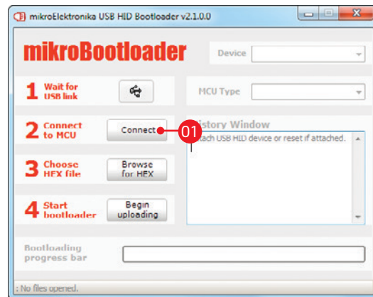
Figure 3-2: USB HID mikroBootloader window
