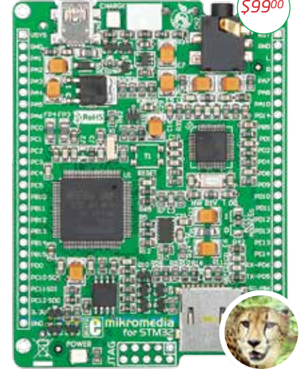
mikromedia for STM32 (features STM32F207VGT6 or STM32F407VGT6)
