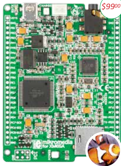
mikromedia for XMEGA (features ATXMEGA128A1)
