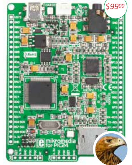
mikromedia for PIC24 (features PIC24FJ256GB110)
