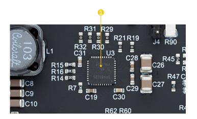
The DRV8323 integrates three bidirectional current sense amplifiers for monitoring the current level through each of the external half-bridges using a low-side shunt resistor. The gain setting of the current sense amplifier can be adjusted through the SPI or hardware interface. The SPI method provides additional flexibility to adjust the output bias point.
