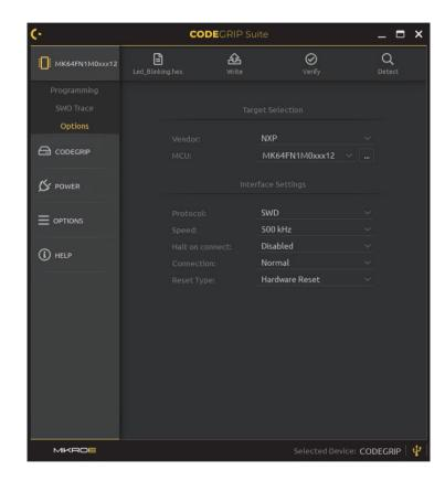
**NOTE** To use the SWO Tracing, the programming protocol must be set to SWD. Not all ARM® MCUs support the SWO Trace. For more information about the SWO Trace capabilities, please consult the datasheet or the reference manual of the used MCU.
