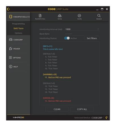
SWO [Serial Wire Output] trace is used to display various SWO-related messages in the Menu item section of the CODEGRIP Suite. The ARM SWO trace port uses a single pin to stream out data packets over 32 different ports, using the specified clock rate. The SWO is a part of the ARM® CoreSight Debug module which is incorporated in most of the MCUs based
