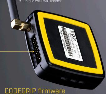
The CODEGRIP device is equipped with the target MCU connector, which contains ICSP/EJTAG and power supply pins. This connector is used to interface the CODEGRIP device with the target MCU, allowing it to perform programming and debugging operations, to provide the power supply for the target MCU, and to be used as the power input when the CODEGRIP device is powered from the connected development board.
