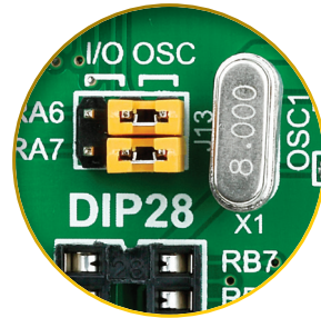
Figure 12: RA6 and RA7 connected to X1 quartz-crystal
