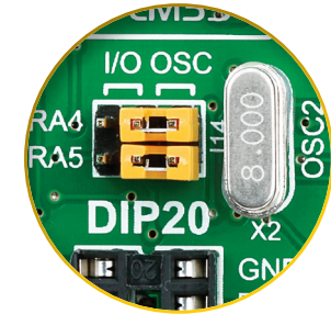
Figure 14: RA4 and RA5 connected to X2 quartz-crystal
