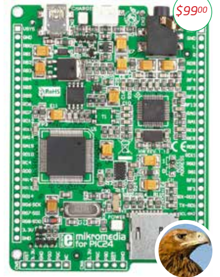
mikromedia for PIC24 (features PIC24FJ256GB110)
