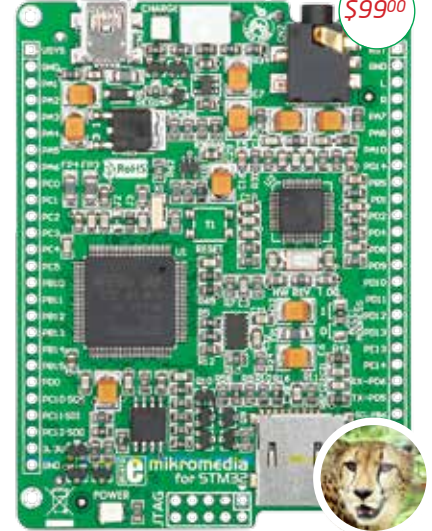
mikromedia for STM32 (features STM32F207VGT6 or STM32F407VGT6)
