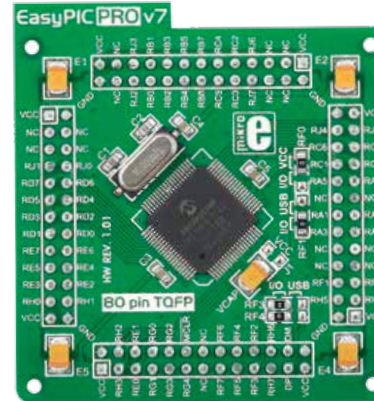
3 Figure 4-7: Standard 80-pin MCU card with PIC18F8722 .
