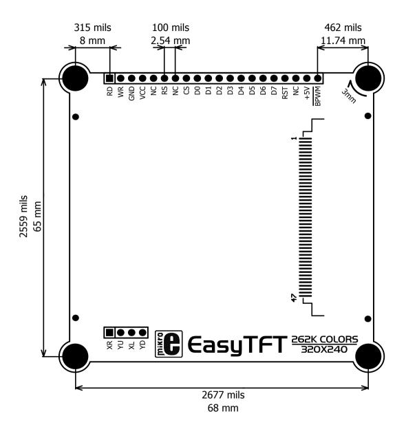
Figure 3: EasyTFT board dimensions.
