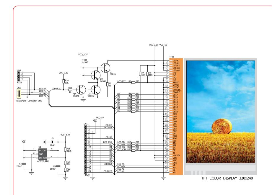
Figure 2: EasyTFT board schematic
