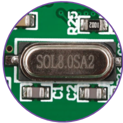
Figure 5-1: External crystal oscillator (X1)
