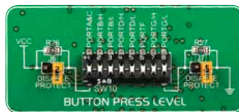
Figure 6-5: Button press level DIP switch (tri-state)
