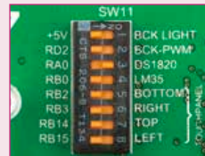
Figure 20-3: Enabled SW11.3 DIP switch
