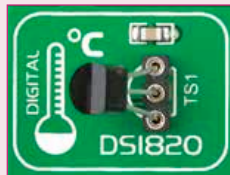
Figure 20-2: DS1820 correctly placed in socket
