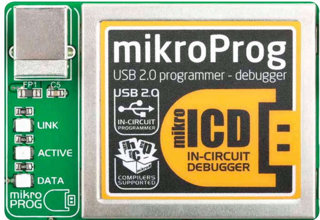
Figure 5-1: mikroProg™ is well protected under metal casing
