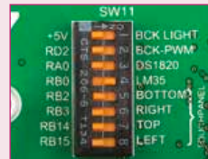
Figure 21-3: Enabled SW11.4 DIP switch
