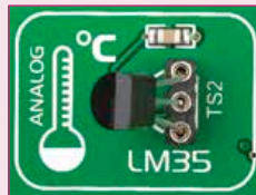
Figure 21-2: LM35 correctly placed in socket
