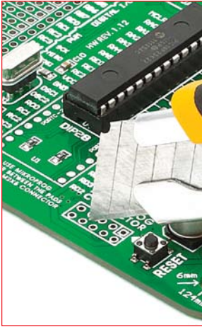
Figure 3-2: cutting copper between pads
