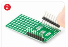
Turn the board upside down so that bottom side is facing you upwards. Place shorter parts of the header pins in both soldering pad locations.
