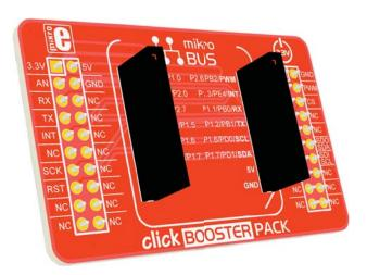
Click BOOSTER PACK is the add-on board for LaunchPad® from Texas Instruments<sup>®</sup>. It features mikroBUS™ host socket, allowing developers to use dozens of click™ add-on boards from mikroElektronika.
