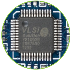
Figure 8-1: On-board VS1053 MP3 codec
