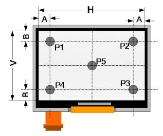
FIG.3. The definition of viewing angle
