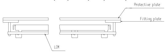
(2) When assembling the LCM into other equipment, the spacer to the bit between the LCM and the fitting plate should have enough height to avoid causing stress to the module surface, refer to the individual specifications for measurements. The measurement tolerance should be  $\pm 0.1 \, \text{mm}$ .
