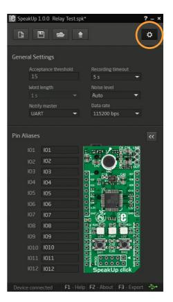
Noise level: Minimal sound volume level that can trigger a voice command recognition. Lower values require quieter pronunciation, resulting in higher noise/hiss sensitivity. On the contrary, higher level values require louder pronounciation and they are less sensitive to noise/hiss.
