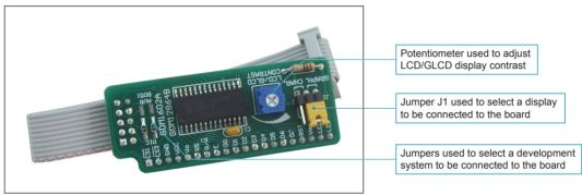
Figure 1: Serial LCD/GLCD Adapter additional board
