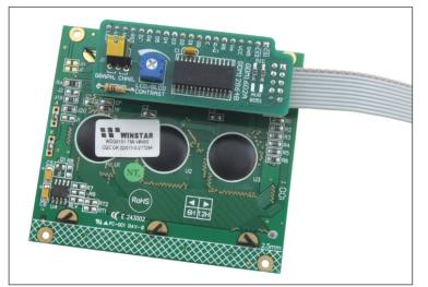
Figure 5: Serial LCD/GLCD Adapter additional board with a 128x64 GLCD (jumper J1 in GRAPH position)
