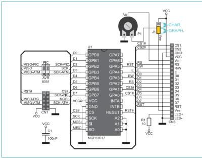
Figure 7: Serial LCD/GLCD Adapter additional board connection schematic
