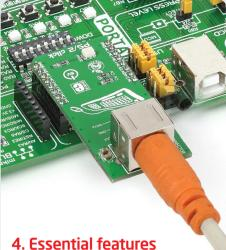
Even though somewhat superseded by USB, PS/2 connectors are still used. PS/2 click™ is especially suited for connecting vintage or certain modern high-end keyboards and mice. One of the key benefits of PS/2 is that it supports full n-key rollover. It's the ability of the keyboard to handle any number of simultaneous keystrokes.
