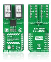
Hall current click<sup>™</sup> is a high precision current sensor. It carries a galvanically isolated TLI4970-D050T4 miniature magnetic digital current sensor that utilizes the Hall effect to measure electric current. The board carries two EXTreme ZPower connectors to connect the conductor. The sensor readings are sent to the target board through the **mikroBUS**<sup>™</sup> SPI (SDO, SCK, and CS) lines. The board uses a 3.3V power supply only.
