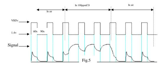
signal when the sensor is shifted from clean air to carbon monoxide (CO), output signal measurement is made within one or two complete heating period (2.5 minute from high voltage to low voltage).
