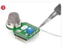
Turn the board upward again. Make sure to align the headers so that they are perpendicular to the board, then solder the pins carefully.
