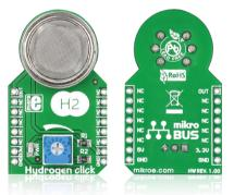
for adding a high sensitivity hydrogen (H<sub>2</sub>) sensor to your design. It's suitable for designing gas leakage equipment. The board features an MQ-8 sensor, a calibration potentiometer, a **mikroBUS**™ socket and a power indicator LED. Hydrogen click<sup>™</sup> communicates with the target board through mikroBUS<sup>™</sup> AN (OUT) line. Hydrogen click<sup>™</sup> is designed to use a 5V power supply only.
