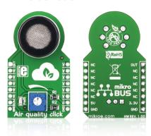
Air quality click<sup>™</sup> is a simple solution for adding a high sensitivity sensor for detecting a variety of gases that impact air quality in homes and offices. The board features an MQ-135 sensor, a calibration potentiometer, a mikroBUS<sup>™</sup> host socket, two jumpers and a power indicator LED. Air quality click<sup>™</sup> communicates with the target board through mikroBUS<sup>™</sup> AN (OUT) line. Air quality click<sup>™</sup> is designed to use a 5V power supply only.
