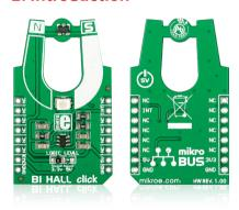
BI HALL click<sup>™</sup> is a simple solution for adding a bipolar Hall switch to your design. It carries the Melexis US2882 bipolar Hall-effect switch and a 74LVC1T45 single bit, dual supply transceiver. BI HALL click<sup>™</sup> communicates with the target board through the mikroBUS<sup>™</sup> INT line. The board is designed to use either a 3.3V or 5V power supply (which also defines the logic level of the output signal).
