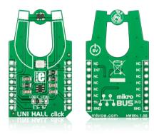
UNI HALL click<sup>™</sup> is a simple solution for adding an unipolar Hall switch to your design. It carries the Melexis US5881 unipolar Hall-effect switch and a 74LVC1T45 single bit, dual supply translating transceiver. UNI HALL click<sup>™</sup> communicates with the target board through the **mikroBUS**<sup>™</sup> INT line. The board is designed to use either a 3.3V or 5V power supply (which also defines the logic level of the output signal).
