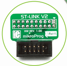
Figure 3-11: mikroProg™ to ST-LINK™ V2 adaper
