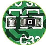
Figure 5-1: zero-ohm J1 jumper
