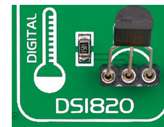
Figure 23-3: DS1820 correctly placed in socket
