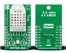
DHT22 click<sup>™</sup> is a temperature and humidity measurement board carrying the AM2302 sensor (also known as DHT22). It's a low cost reliable sensor that communicates with the target board microcontroller through a single Serial Data Line. You can choose between the mikroBUS<sup>™</sup> CS or INT pins for communicating with the target board microcontroller. The board is designed to use either a 3.3V or a 5V power supply.
