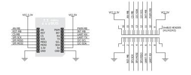
Vertical mikroBUS™ socket schematic
