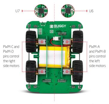
To prevent the motors from drawing too much current from the battery (and in doing so prevent the other components from functioning properly) a few resistors are placed to limit current draw. Each motor can draw a maximum of 400 mA, for a total of 1.6 A for all four motors.
