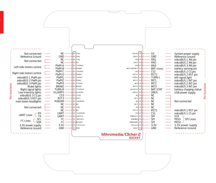
The Buggy carries a standard clicker 2/mikromedia pinout with a pair of 1x26 connection pads. However, to make the Buggy easier to program, some of the pins have descriptive labels that point out their functions in relations to the motors, lights and so on.
