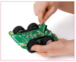
**STEP 7 -** Insert mikroBUS<sup>™</sup> socket plates
