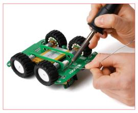
**STEP 8** - Solder mikroBUS<sup>™</sup> socket plates
