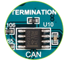
Figure 16-2: CAN transceiver with Node TERMINATION jumper
