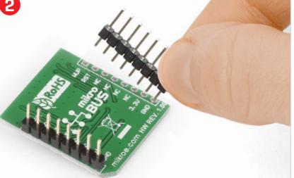
Turn the board upside down so that the bottom side is facing you upwards. Place shorter pins of the header into the appropriate solder pads.
