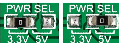
*Nano GPS click* features an SMD jumper [zero ohm resistor] that lets you switch between a 3.3V or a 5V power supply.
