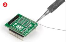
Turn the board upward again. Make sure to align the headers so that they are perpendicular to the board, then solder the pins carefully.
