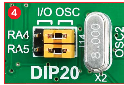
Figure 4-9: RA4 and RA5 connected to X2 quartz-crystal
