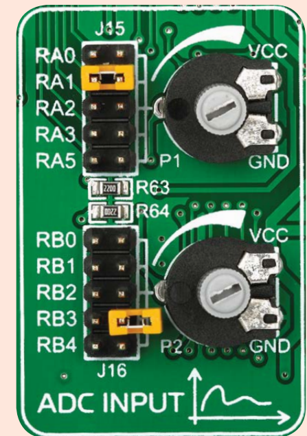
Figure 17-1: use J15 and J16 jumpers to connect analog input lines with potentiometers P1 and P2
