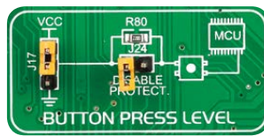
Figure 10-5: Button press level jumper (J17)
