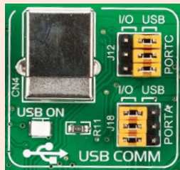
Figure 8-2: USB enabled on PORTC
