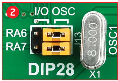
Figure 4-7: RA6 and RA7 connected to X1 quartz-crystal
