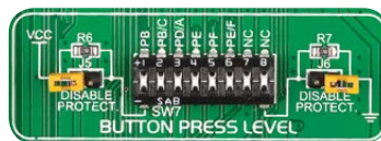
Figure 10-6: Button press level DIP switch (tri-state)
