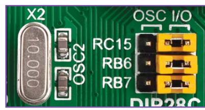
Figure 4-8: RC15, RB6 and RB7 as I/O pins (when using internal oscillator)
