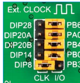
Figure 4-10: Position of the jumpers for DIP8
