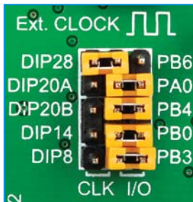
Figure 4-6: Position of the jumpers for DIP28
