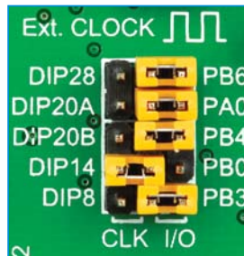
Figure 4-9: Position of the jumpers for DIP14
