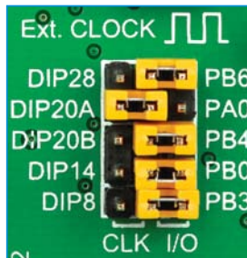
Figure 4-7: Position of the jumpers for DIP20A
