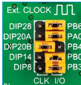
Figure 4-8: Position of the jumpers for DIP20B
