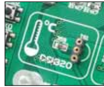
Figure 13-1: DS1820 connector (DS1820 is not placed)
