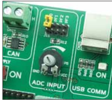
Figure 12-1: ADC (jumper idefault position)
