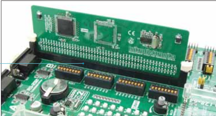
Figure 2-2: DIMM-168P connector with the MCU card inserted
