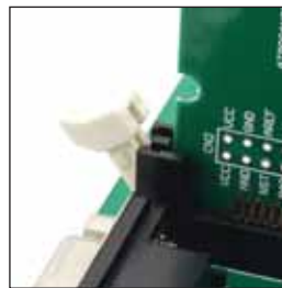
Extraction levers used to fix MCU card in the 'open' position
