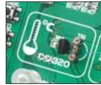
Figure 13-2: DS1820 connector with the DS1820 temperature sensor plugged into
