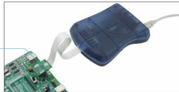
Figure 5-2: JTAGICE mkII connected to the board
