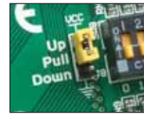
Figure 21-3: J2 in pull-up position
