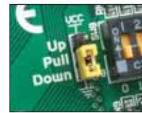
Figure 21-2: J2 in pull-down position
