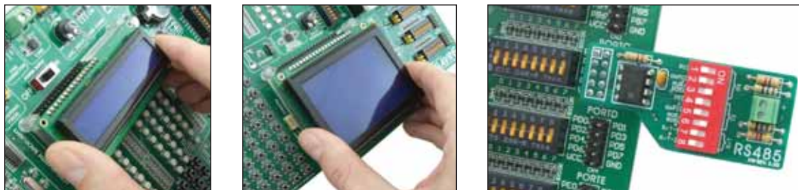
Figure 1-3 : Placing additional modules on the board
