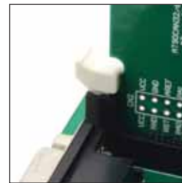
Extraction levers used to fix MCU card in the 'closed' position
