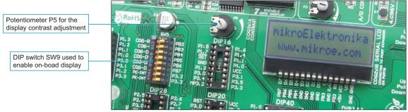
Figure 13-1: On-board 2x16 LCD display
