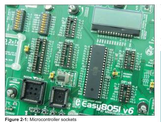
There are two sockets for 8051 microcontrollers in DIP14 package provided on the board. Which of these sockets will you use depends solely on the pinout of the microcontroller in use. The *Easy8051 v6* development system comes with the microcontroller in DIP40 package.
