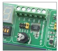
Figure 7-2: Pin CH0 used as A/D conversion input
