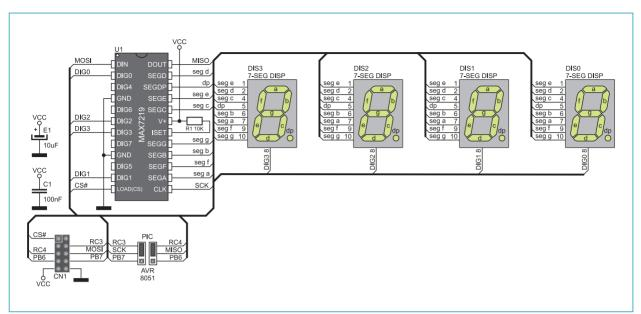
Figure 6: Serial 7-Seg Display additional board connection schematic
