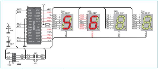
Figure 5: Principle of time-multiplexing performed on the DIS2 display
