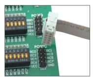
Figure 2: Connecting IDC10 connector
