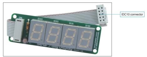
Figure 1: Serial 7-Seg Display additional board
