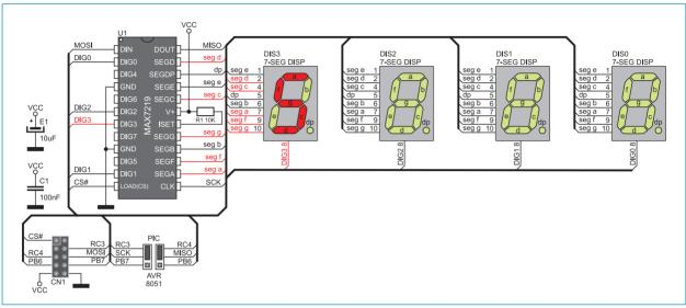
Figure 4: Time-division multiplexing performed on the DIS3 display
