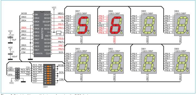
Figure 5: Principle of time-multiplexing performed on the DIS6 display
