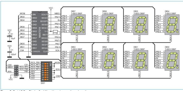
Figure 2: Serial 7-Seg Display 2 additional board connection schematic
