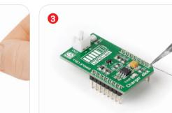
Turn the board upside down so that Turn the board upward again. Make sure the bottom side is facing you upwards. to align the headers so that they are Place shorter pins of the header into the perpendicular to the board, then solder the pins carefully.
