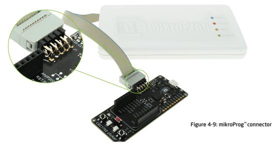
The microcontroller can be programmed with external **mikroProg**<sup>™</sup> for CEC1702 programmer and **mikroProg Suite<sup>™</sup> for ARM**<sup>®</sup> software.
