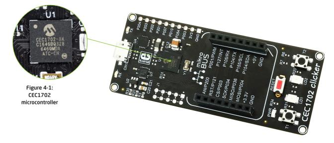
The microcontroller can be programmed using external mikroProg<sup>™</sup> for CEC1702 programmer.
