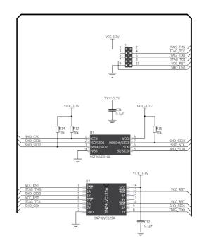
Figure 4-13: mikroProg<sup>™</sup> connection schematic
