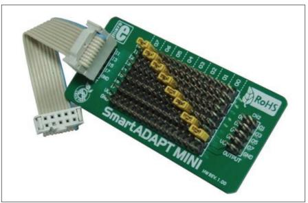
Figure 1: Smart ADAPT MINI additional board
