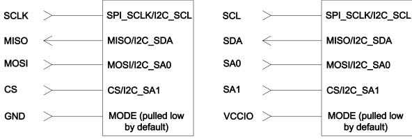
**SPI Interface** – the SPI slave interface operates up to 30MHz.
