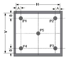
Figure 3.The definition of viewing angle
