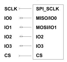
Figure 5. QSPI interface connection
