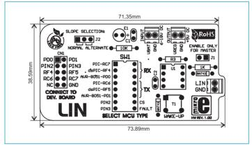
Figure 3: Dimensions of the LIN additional board
