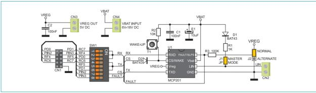
Figure 2: LIN additional board connection schematic
