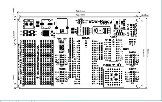
Figure 5: Additional board dimensions
