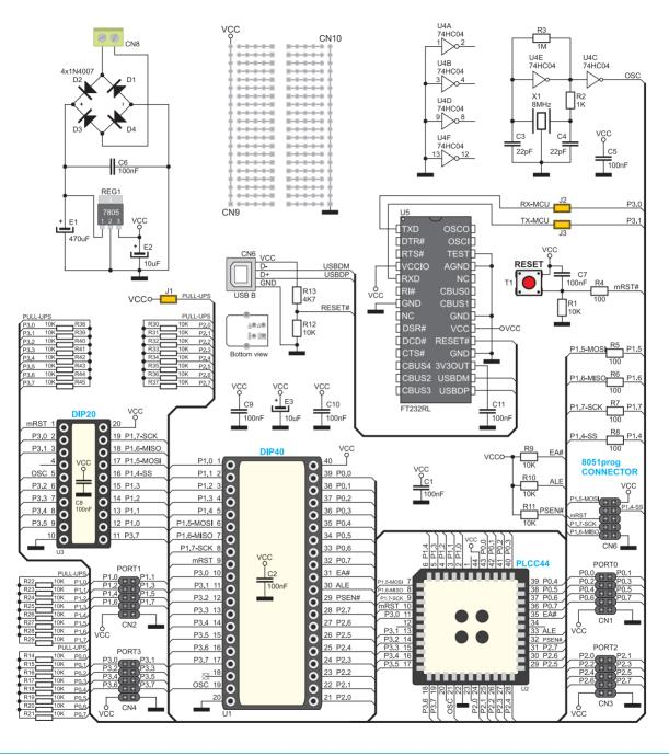
Figure 4: Additional board connection schematics
