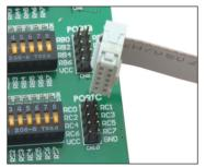
Figure 2: Plugging IDC10 connector into a development system
