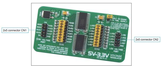
Figure 1: 5V-3.3V VOLTAGE TRANSLATOR additional board
