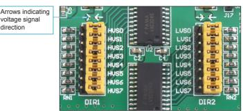
Figure 5: Jumpers DIR1 and DIR2 in the position for 3.3V to 5V voltage level adjustment
