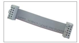
Figure 3: Flat cable with IDC10 connectors
