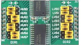
Figure 6: Jumpers DIR1 and DIR2 in the position for bidirectional transfer
