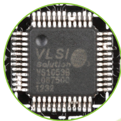
Figure 8-1: On-board VS1053 MP3 codec
