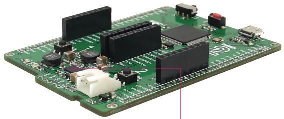
Clicker 2 for PIC32MZ features LTC®3586, a highly integrated power management and battery charger IC that includes a current limited switching PowerPath manager. LTC®3586 also enables battery charging over a USB connection.
