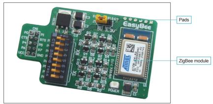
Figure 1: EasyBee additional board
