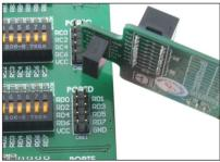
Figure 2: Connecting additional board
